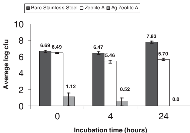
Figure 6. Surviving colony-forming units on bare stainless steel, zeolite A-coated stainless steel, and silver-ion-exchanged zeolite A over a 24 h incubation period.
