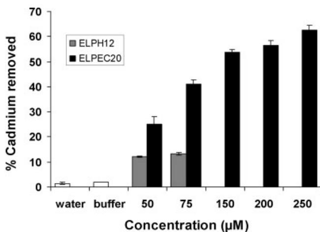
**Figure 6.** The efficiency of batch soil washing by ELPEC20 and ELPH12. Experiments were carried out with 1 g of soil at a constant 1:10 (w/v) soil to solution ratio. The percentage of cadmium removed was calculated based on an initial cadmium content of 296.9 mg/kg.
