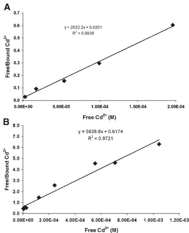
**Figure 3.** Ruzic plots of free Cd ion concentration/bound Cd ion concentration against free Cd ion concentration for ELPEC20 (A) and ELPH12 (B). The cadmium binding constant was calculated by dividing the y-intercept by the slope for the linear plot.
