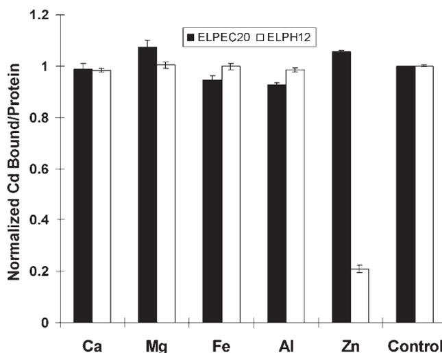
**Figure 4.** Cadmium binding by ELPH12 and ELPEC20 in the presence of other divalent cationic metals. In the control experiment, 100  $\mu\text{M}$  of  $\text{Cd}^{2+}$  and biopolymers were added. For the competitive binding experiments, 100  $\mu\text{M}$  of the corresponding metal was also added.
