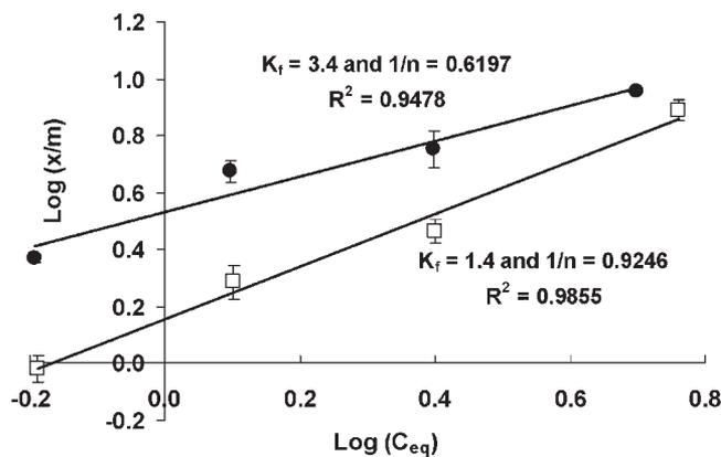
**Figure 5.** Comparison of Freundlich isotherms for adsorption of ELPEC20 (●) and ELPH12 (□) onto soil.  $x$  is the amount of ELP biopolymer adsorbed (mg),  $m$  is the mass of soil (g), and  $C_{eq}$  is the concentration of biopolymer (mg/mL) remaining in solution after adsorption.
