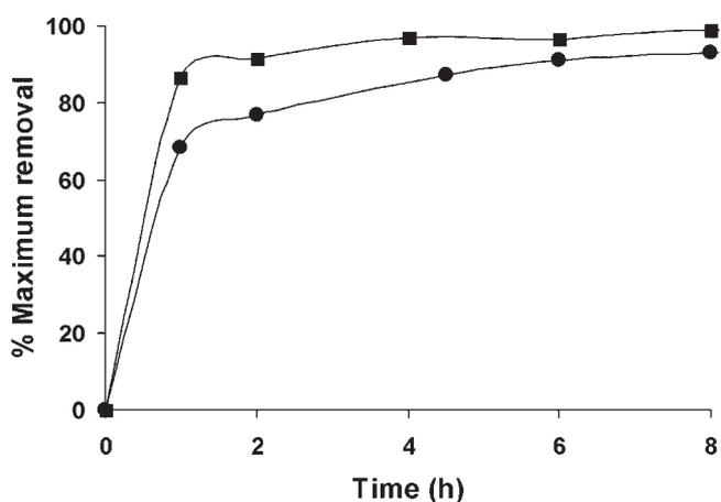
**Figure 7.** The kinetics of cadmium extraction by ELPEC20 (■) and ELPH12 (●).
