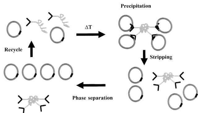
**Figure 1.** Principle of the affinity purification of plasmid DNA based on temperature-triggered precipitation of ELP biopolymers.
