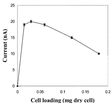
Fig. 2. Effect of cell loading on biosensor response to 5  $\mu\text{M}$  PNP in 50 mM pH 7.5 citrate-phosphate buffer at room temperature. Operating potential: +0.4 V (vs. Ag/AgCl). Data are given as mean  $\pm$  1 SD for three experiments.
