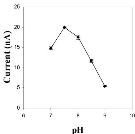
Fig. 3. Effect of pH (50 mM citrate-phosphate) on biosensor response to 5  $\mu\text{M}$  PNP with 0.03 mg cell loading at room temperature. Operating potential: +0.4 V (vs. Ag/AgCl). Data are given as mean  $\pm$  1 SD for three experiments.
