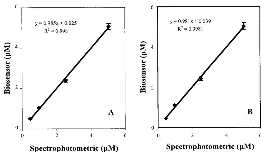
Fig. 5. Accuracy of amperometric microbial biosensor. A) in 50 mM pH 7.5 citrate-phosphate buffer and B) in Lake Elsinore water filtered and adjusted to pH 7.5, at room temperature with 0.03 mg cell loading, applying +0.4 V to working electrode vs. the Ag/AgCl reference. Data are given as mean  $\pm$  1 SD for three experiments.
