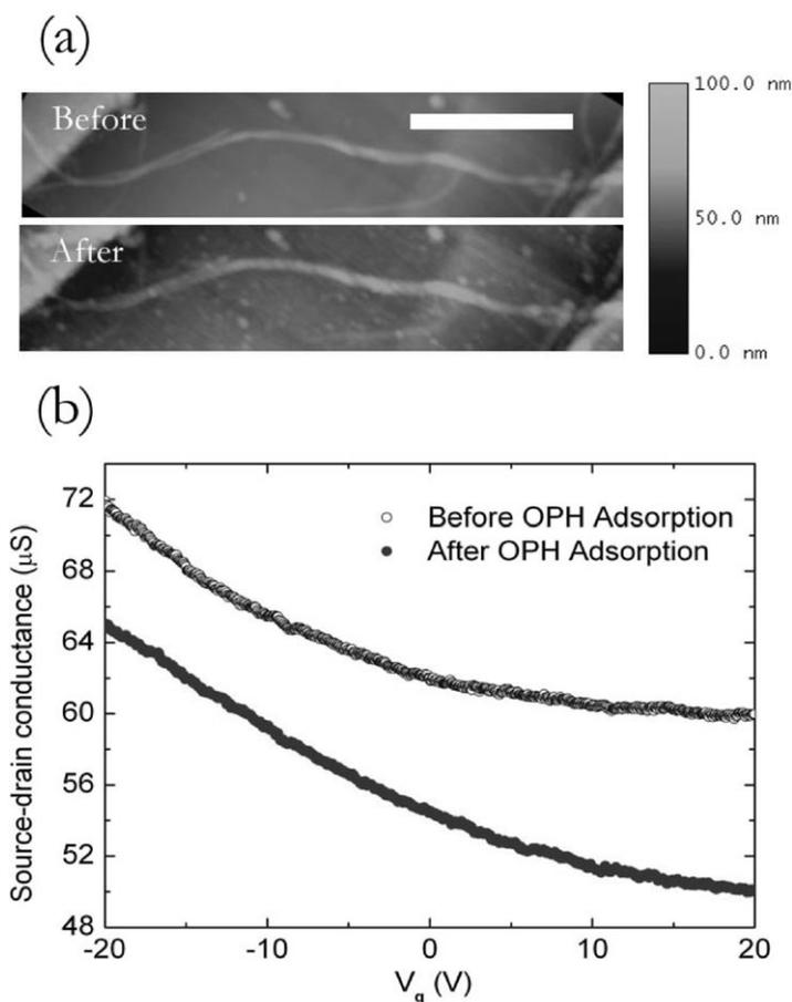
Fig. 2. a) AFM images of a typical SWNT sensor before and after OPH immobilization. The scale bar is 1  $\mu\text{m}$ . b)  $I-V_g$  curves of the SWNT sensor before and after OPH immobilization.
