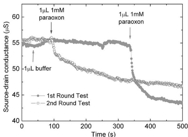
Fig. 4. The response of another OPH functionalized SWNT sensor to phosphate buffer and paraoxon. After the first round test, the device was rinsed and blown dry with nitrogen. Before the second round real-time measurement, 1  $\mu\text{L}$  phosphate buffer was used to wet the SWNT channel. The p-type silicon was connected to ground.
