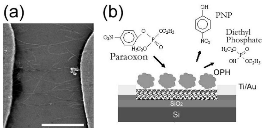
Fig. 1. a) SEM picture of a typical SWNT sensor. Well aligned SWNT networks connect the electrodes. The scale bar is 1  $\mu\text{m}$ . b) Schematic of paraoxon detection based on an OPH functionalized SWNT electronic sensor.
