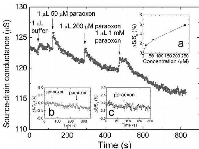
Fig. 3. Real-time response of an OPH functionalized SWNT sensor to phosphate buffer and different concentrations of paraoxon. The SWNT channel of the sensor was immersed in 1  $\mu\text{L}$  buffer initially. The p-type silicon was connected to ground. Inset (a) shows relative conductance change of the device as a function of OP concentration. Inset (b) shows the response of a device with inactive OPH. Inset (c) shows the response of as-prepared CNTFET without OPH to paraoxon.
