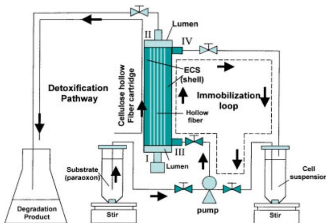
**Figure 1.** Schematic diagram of the hollow fiber bioreactor system. [Color figure can be seen in the online version of this article, available at [www.interscience.wiley.com](http://www.interscience.wiley.com).]
