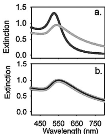
**Fig. 3** UV-vis extinction spectra of an active 17E DNAzyme-nanoparticle sensor (a) and an inactive 17Ec DNAzyme-nanoparticle sensor (b) in the absence (light grey curve) or in the presence (dark grey curve) of 5  $\mu\text{M}$  Pb(II).<sup>107</sup>
