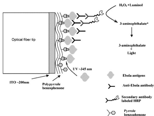
**Fig. 5** The biosensor scheme describing the various steps involved in the immunoassay using ITO–poly(pyrrole-benzophenone)-coated optical fibers for the detection of anti-Ebola virus in sera samples.<sup>121</sup>
