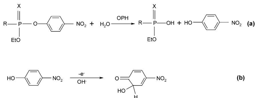
**Scheme 2** (A) Reaction scheme of the OPH catalyzed hydrolysis of parathion, methyl parathion and paraoxon. (B) Electrochemical oxidation of *p*-nitrophenol. Parathion: X = S, R = ethoxy; methyl parathion: X = S, R = methoxy; paraoxon: X = O, R = ethoxy
