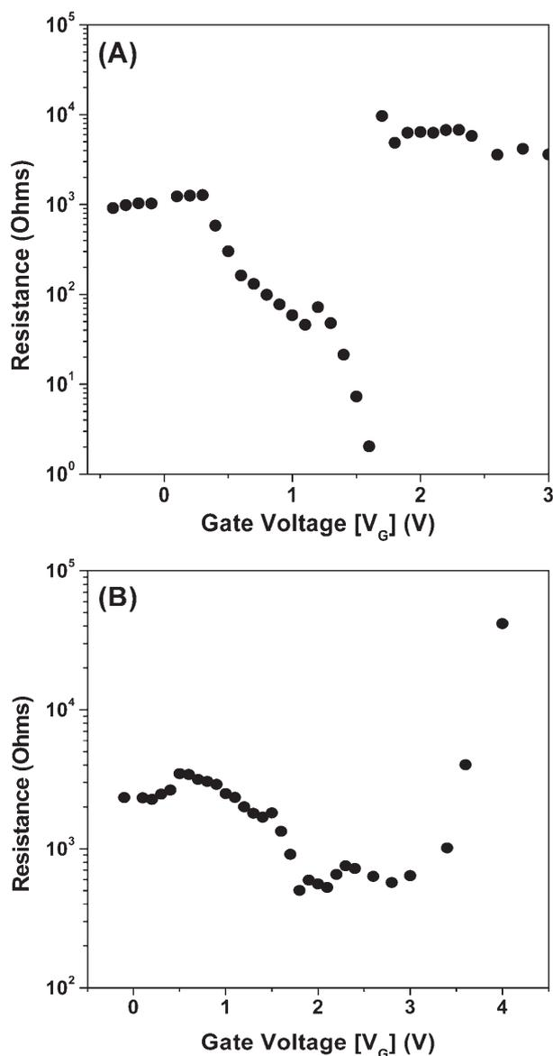
Fig. 7. A) Resistance vs. gate voltage of PPY/Cl film in 0.1 M aqueous NaCl. B) Resistance vs. gate voltage of PPY/SWNT-PABS film in 0.1 M aqueous NaCl.
