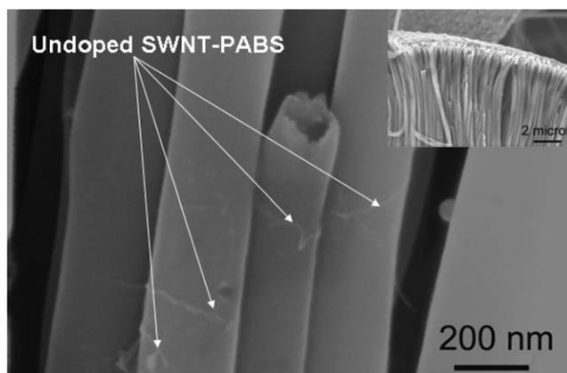
Fig. 9. SEM images of PPY/SWNT-PABS nanotubes. Inset: A low resolution SEM image of bundle of nanotubes.
