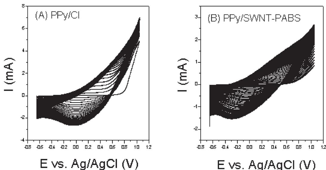
Fig. 2. Cyclic voltammograms of the film growth of PPy/SWNT-PABS and PPy/Cl. Electrolyte: 0.25 M aqueous pyrrole containing 0.09 mg/mL SWNT-PABS. Scan rate: 50 mV/s, 50 cycles.
