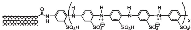
Fig. 1. Chemical structure of SWNTs functionalized with PABS.
