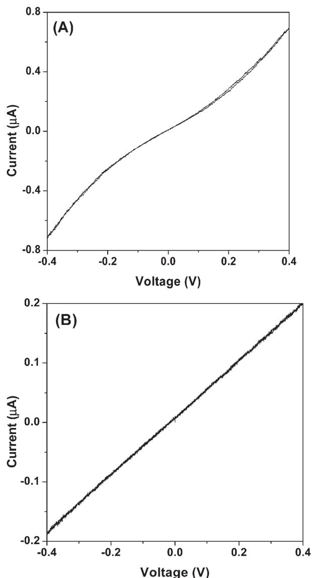
Fig. 6.  $I-V$  characteristics of PPy/Cl (A) and PPy/SWNT-PABS (B) films. Electrolyte = 0.1 M NaCl, scan rate = 50 mV/s.
