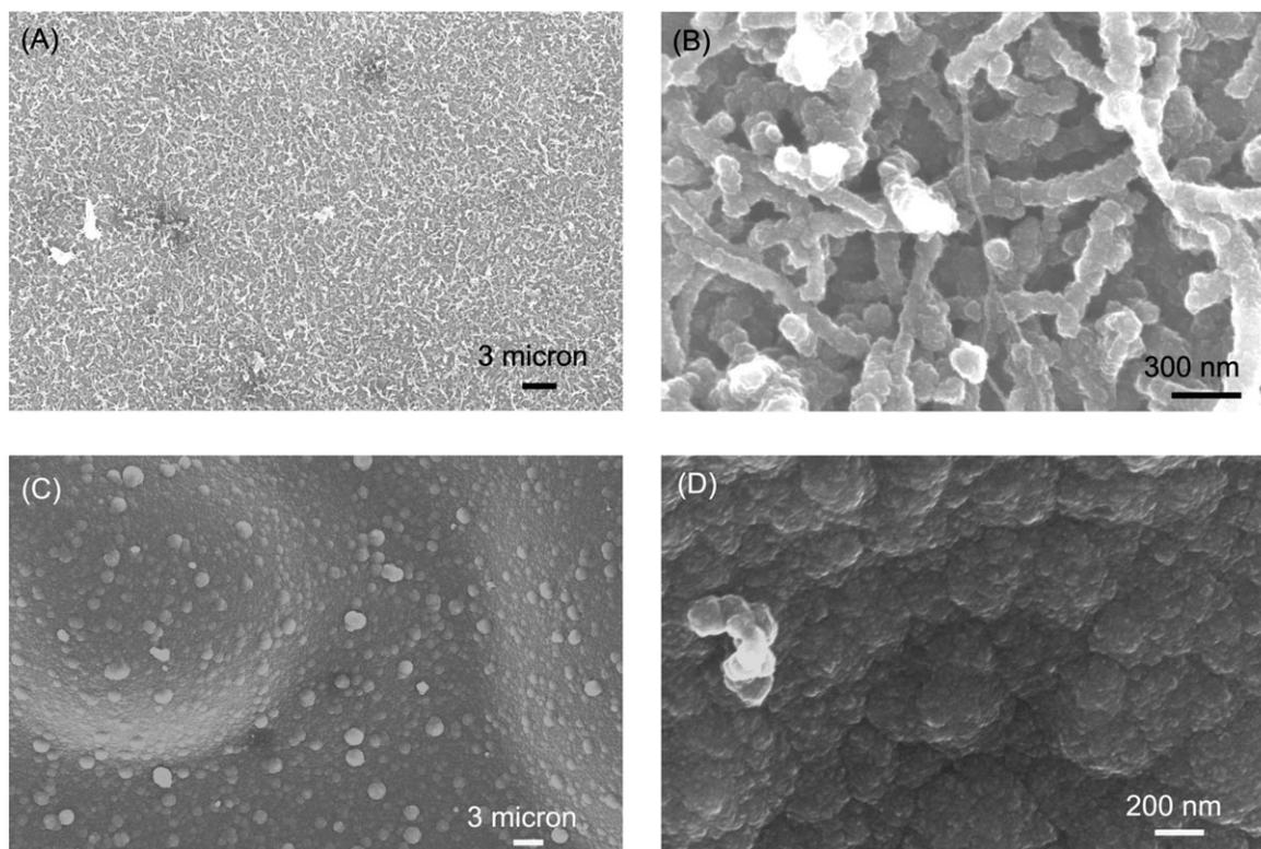
Fig. 4. SEM images PPY/SWNT-PABS film (A and B) and PPY/Cl film (C and D).
