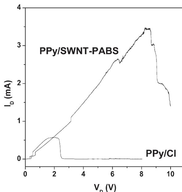
Fig. 8. Breakdown voltage of PPY/Cl and PPY/SWNT-PABS films in air. Scan rate = 200 mV/s.
