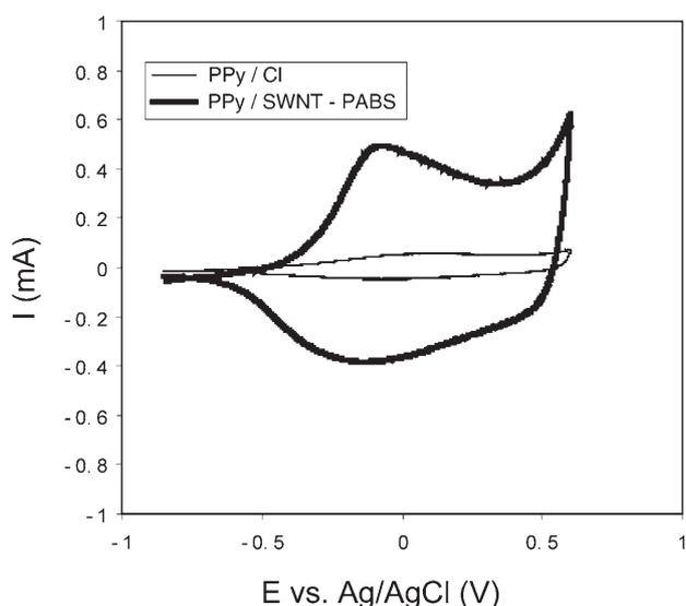
Fig. 3. Cyclic voltammograms for the comparison of PPy/SWNT-PABS composite film and PPy/Cl<sup>-</sup> film prepared under same conditions. Scan rate 50 mV/s, electrolyte 0.5 M NaCl.
