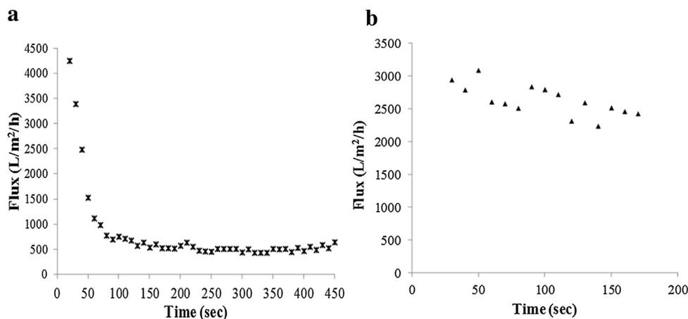
**Fig. 8.** Permeate flux during ELP-Z precipitate recovery using NFF. (a) Permeate flux during the 5 μm filtration of the ELP-Z precipitate feed and (b) Permeate flux during the 0.45/0.2 μm filtration of the permeate stream from the 5 μm filtration step.
