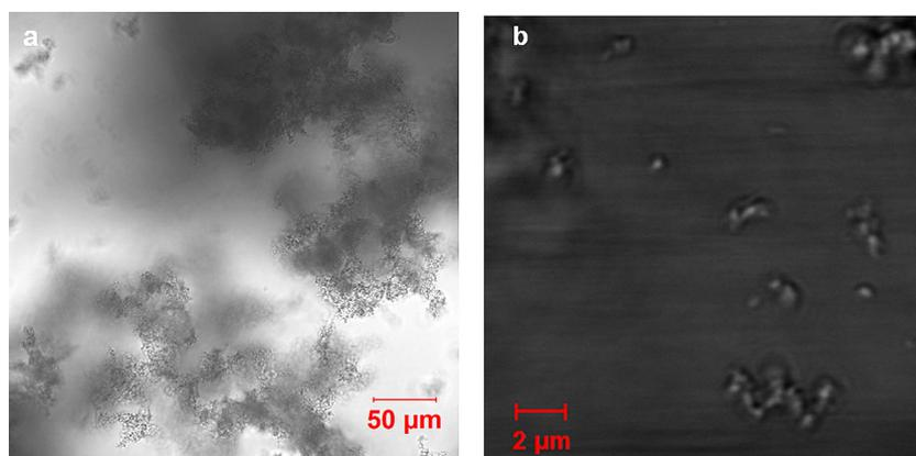
**Fig. 6.** ELP-Z-mAb complex precipitates bright field image for 4:1 ELP-Z:mAb molar ratio after 10 min. (a) Scale bar 50  $\mu\text{m}$  and (b) higher resolution image, scale bar 2  $\mu\text{m}$ .
