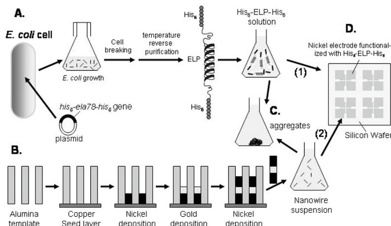
**Figure 1.** A schematic diagram depicting the strategies applied in this paper: (A) generation and purification of biopolymer His<sub>6</sub>-ELP-His<sub>6</sub>; (B) Ni/Au/Ni nanowire production; (C) aggregation of Ni/Au/Ni nanowires upon interaction with biopolymers; (D) deposition of Ni/Au/Ni nanowires onto nickel electrodes by biopolymers.
