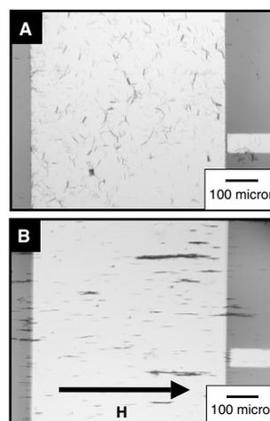
**Figure 4.** Optical micrographs of Ni/Au/Ni nanowires deposition onto peptide-functionalized electrode surfaces in the absence (A) or presence (B) of an external magnetic field in-plane to the electrodes (indicated by an arrow).
