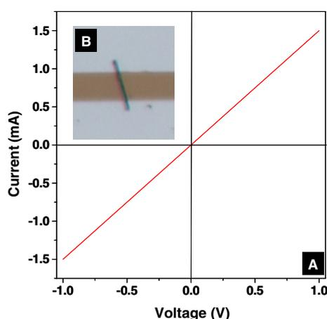
**Figure 6.** A current versus voltage ( $I$ - $V$ ) curve of a single Ni/Au/Ni nanowire bridging two nickel electrodes at a  $50 \text{ mV s}^{-1}$  scan rate. The inset is an optical image of the bridging Ni/Au/Ni nanowire.
