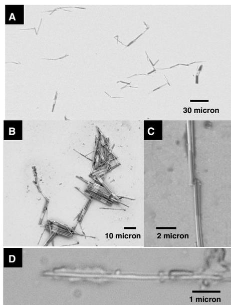
**Figure 2.** SEM images showing the dispersed Ni/Au/Ni nanowires (A) and the assembled nanostructures of nanowires by His<sub>6</sub>-ELP-His<sub>6</sub> biopolymers ((B) and (C)), and an optical image demonstrating the specific interaction between the Ni segments and the His<sub>6</sub>-ELP-His<sub>6</sub> biopolymers (D).
