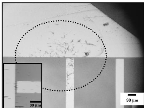
**Figure 5.** An optical micrograph of the site-specific deposition of nanowires. Area exposed to  $0.1 \mu\text{l}$  of His<sub>6</sub>-ELP-His<sub>6</sub> solution was highlighted by a circle. Bridging of electrodes by nanowires using an applied magnetic field is shown in the inset.
