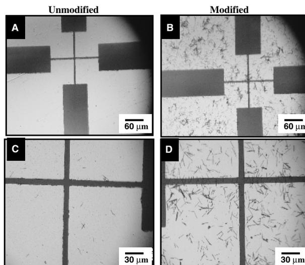
**Figure 3.** Optical micrographs of Ni/Au/Ni nanowires deposition onto unmodified ((A) and (C)) and modified ((B) and (D)) nickel electrodes.
