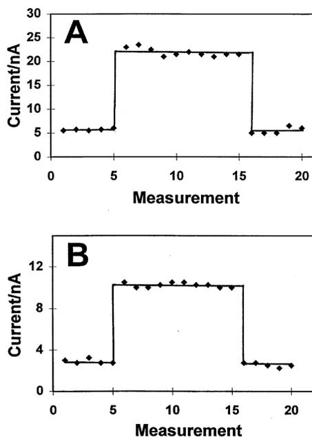
Fig. 2. Carry over experiments. Untreated river water samples, containing  $4.6 \times 10^{-6}$  M and  $23.0 \times 10^{-6}$  M paraoxon (A) or  $1.5 \times 10^{-6}$  M and  $7.5 \times 10^{-6}$  M methyl parathion (B). Other conditions, as in Figure 1.
