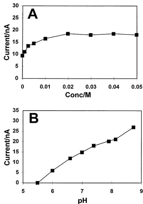
Fig. 4. Effect of solution conditions, including buffer concentration (A) and pH (B) upon the response to  $2.3 \times 10^{-5}$  M paraoxon. Potential step to +0.85 V; medium: phosphate buffer of pH 7.4 (A) and 0.05 M concentration (B).
