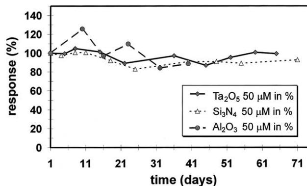
Fig. 8. Comparison of the long-term stability of the three different enzyme biosensors with the transducer materials  $\text{Si}_3\text{N}_4$ ,  $\text{Al}_2\text{O}_3$  and  $\text{Ta}_2\text{O}_5$ . For each sensor, the first measurement was defined as 100% response.
