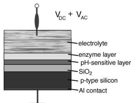
Fig. 1. Capacitive EIS biosensor with immobilised enzyme layer on a pH-sensitive transducer structure (schematically).
