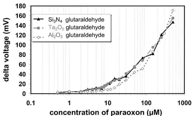
Fig. 7. Influence of the calibration plot towards paraoxon of the enzyme biosensor on the pH-transducing layer used ( $\text{Si}_3\text{N}_4$ ,  $\text{Al}_2\text{O}_3$  and  $\text{Ta}_2\text{O}_5$ ). Each data point represents the mean value of three measuring points for paraoxon concentrations above 15  $\mu\text{M}$ , and the mean value of five measuring points of concentrations below 15  $\mu\text{M}$ . The error bars represent  $\pm 1$  standard deviation.
