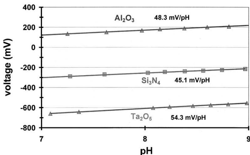
Fig. 4. The pH sensitivity of the EIS biosensor after enzyme immobilization. Al<sub>2</sub>O<sub>3</sub>, Ta<sub>2</sub>O<sub>5</sub> and Si<sub>3</sub>N<sub>4</sub> serve as transducer materials.
