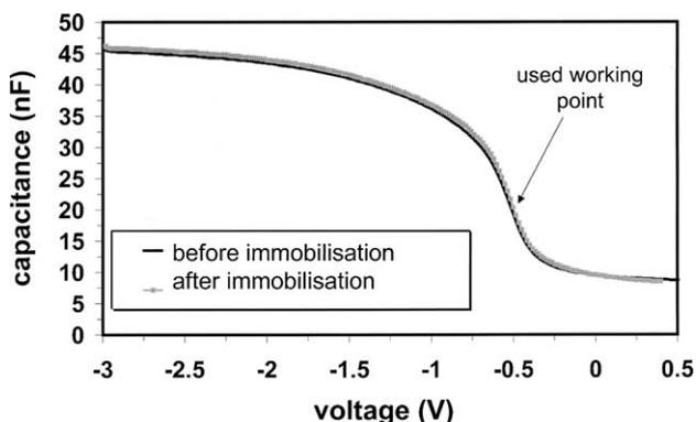
Fig. 3. Capacitance/voltage ( $C/V$ ) curve of a capacitive field-effect sensor with  $\text{Si}_3\text{N}_4$  as pH-sensitive material before (full line) and after enzyme immobilization (open squares) via glutaraldehyde.
