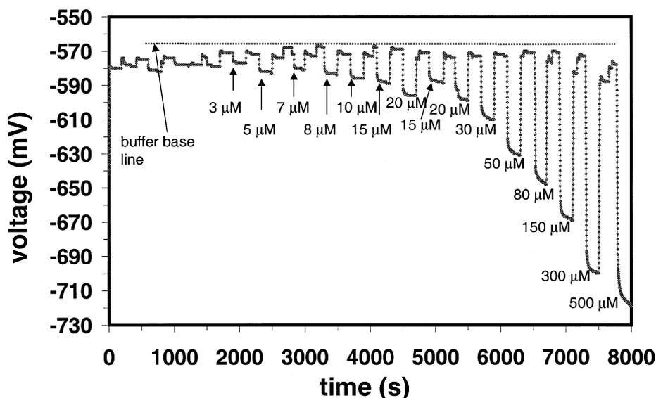
Fig. 5. Typical constant capacitance (ConCap) plot vs. time of the EIS biosensor. The dotted line corresponds to the buffer concentration that is alternatingly measured with the increasing paraoxon concentration.
