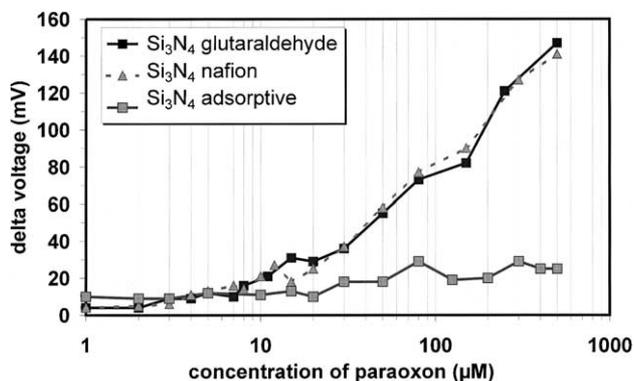
Fig. 6. Calibration curve of the enzyme biosensor for paraoxon with  $\text{Si}_3\text{N}_4$  as pH-sensitive transducer. The enzyme OPH was immobilised by adsorptive-, nafion- and glutaraldehyde coupling.
